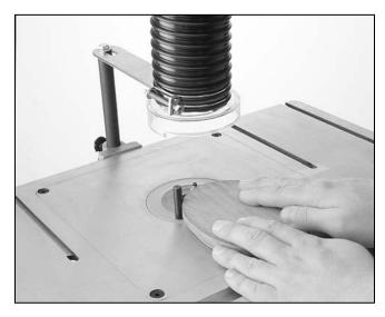
**Figure 25.** Using the starting pin. Note: safety guard has been raised to demonstrate pin positioning.
